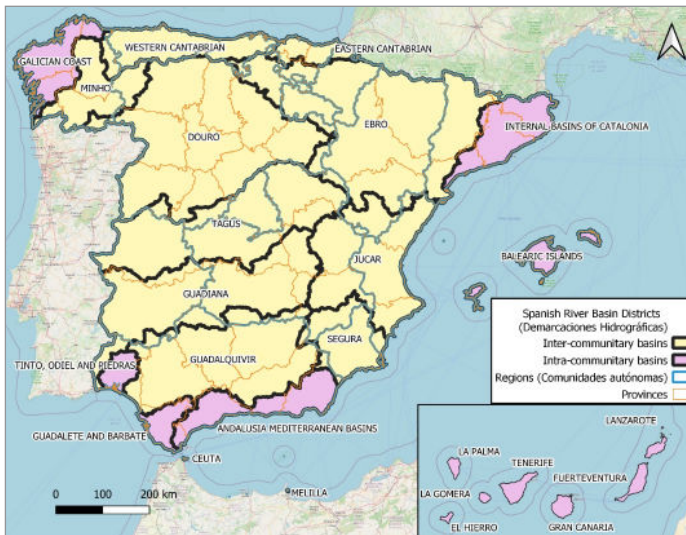
Figure 1. Spanish River Basin Districts. Inter-communitary basins (yellow) are those covering more than one region (comunidad autónoma), and managed by a River Basin Authority (Confederación Hidrográfica). Intra-communitary basins (pink) are located entirely within one region and are managed by the corresponding regional government. Source: Author's elaboration with data from MITERD 15 .
